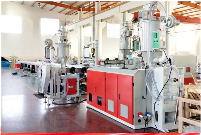
This line is used to produce three layer EVOH oxygen barrier floor heating pipes, such as PEX/EVOH and PERT/EVOH pipes.
